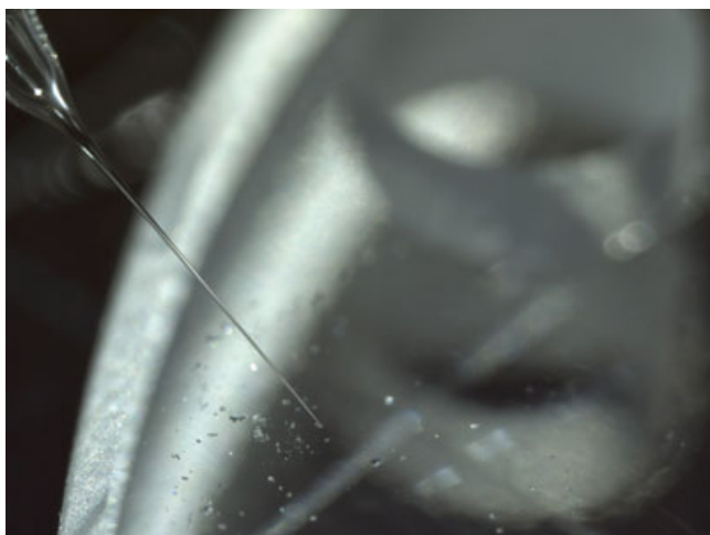
Fig. 12. An optical microscopic image of RA-QD02-0070 picked up with the micromanipulator from the quartz glass disk of catcher room A. This image was taken by the microscope observing the samples from 45° angle. The particle looks translucent in the image.
